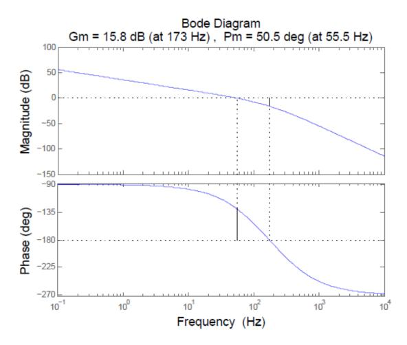
Figure 5.15: Loop Gain and Phase Response of the Dominant Pole Compensated System with Zero
