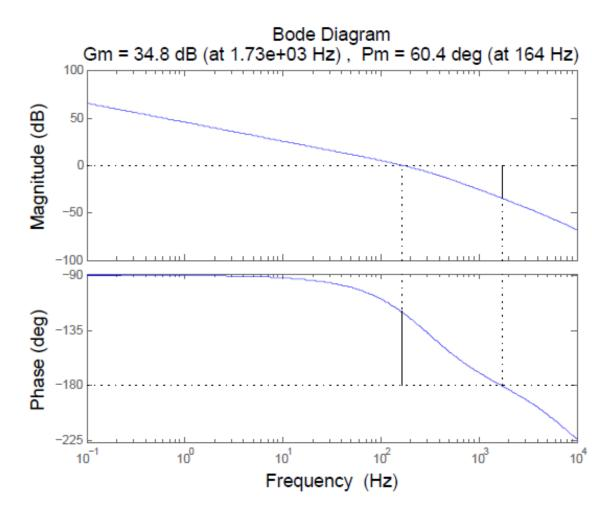
Figure 5.24: Matlab Analysis of Lead Compensated System with integrator and zero
