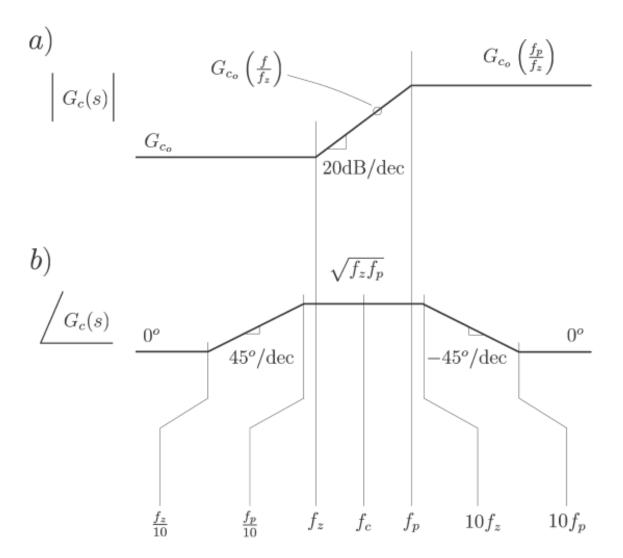
Figure 5.19: Bode Diagram: Lead Compensator
