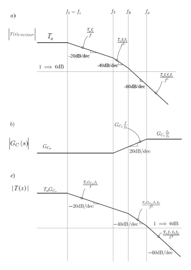
Figure 5.20: Lead Compensation Magnitude Construction
