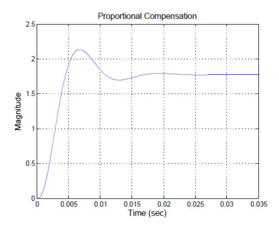
Figure 5.6: Step Response of Proportional Compensated Closed-Loop System
