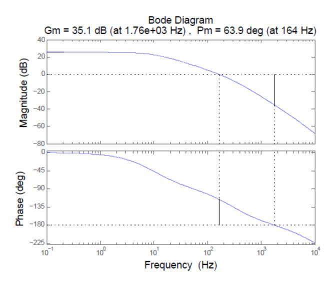
Figure 5.22: Matlab Analysis of Lead Compensated System
