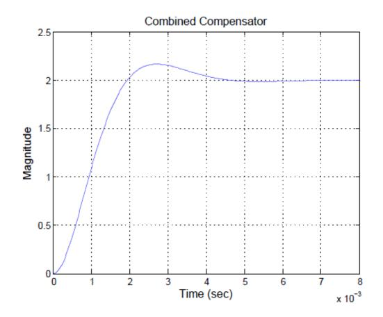
Figure 5.25: Step Response of the Lead Compensated System with integrator and zero
