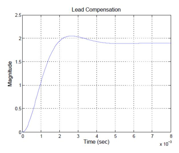
Figure 5.23: Step Response of the Lead Compensated System
