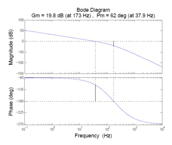
Figure 5.17: Matlab Analysis of Dominant Pole Compensated System with Zero (Improved Margin)
