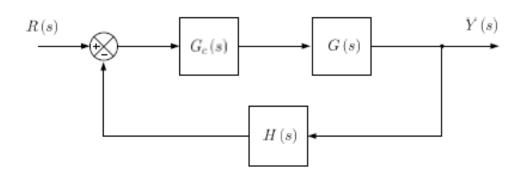
Figure 5.1: Feedback System Block Diagram
