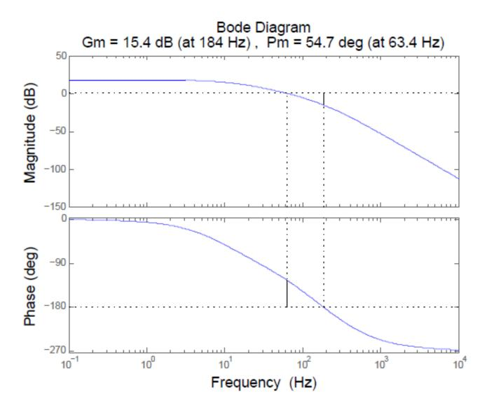
Figure 5.5: Matlab Proportional Compensated Loop Gain Bode Plot
